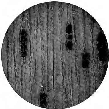
398. Longitudinal tangential section of Scotch pine wood, highly magnified. It shows tracheids with bordered pits. The dark cells are ends of medullary rays.
