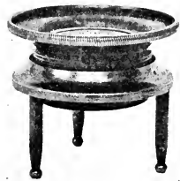
FIG. 72.—A cheap magnifier well adapted for use in analyzing seeds. The magnifier is set over the seeds, leaving the hands free to separate the seeds as one looks through the magnifier from above.
