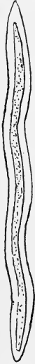
FIG. 116.—A wood fiber, consisting of a much elongated cell with thick walls.
