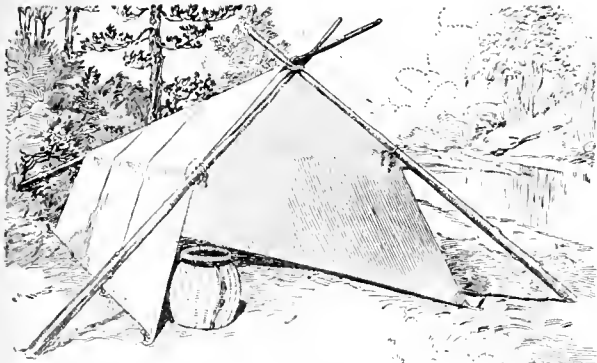
The Forester's Tent is Quickly Erected by Using Three Small Saplings. One along the Ridge, and One on Each Side of the Opening to Form a Crotch for the Ridge Pole
