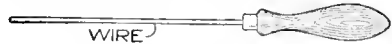
The Tool will Pick Up a Drop of Oil and Deposit It Where Wanted
