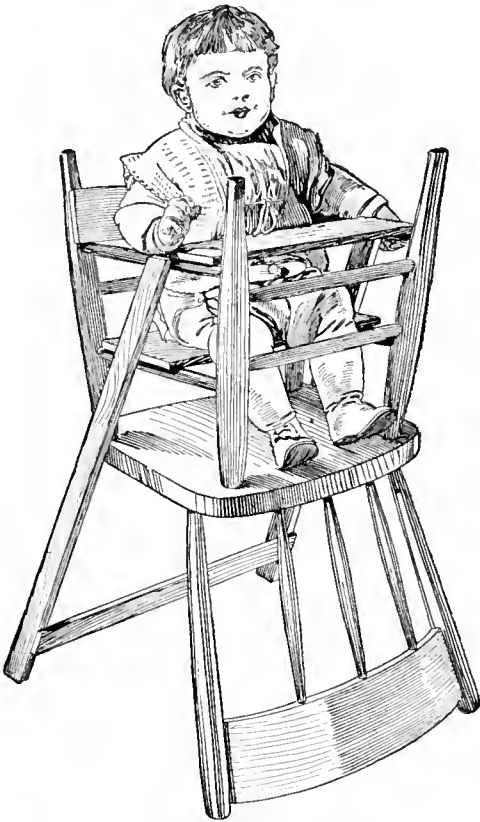
An Inverted Solid-Bottom Chair with Attachments Used for a Child's High Chair
