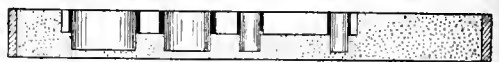
A Mold Made in Plaster without a Special Pattern and Run with a Soft Metal
