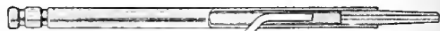
AIR SUPPLY— Blowpipe Connection to the Ordinary Illuminating-Gas Main for Hard and Soft Soldering
