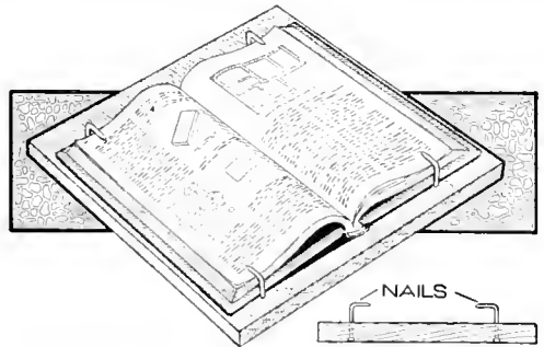
Nails Driven in a Board and Bent in the Shape of Screw Hooks to Hold a Book
