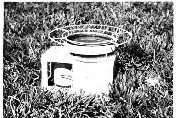
Fig. 5. Evaporimeter for daily measurement of potential evaporation.
