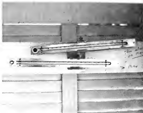
Fig. 7. Maximum and minimum thermometers located in a standard weather shelter.
