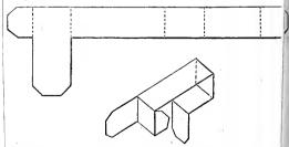
it has to be folded. It can be folded on a hard wood or metal stock just the size of the top bar of the frame. When folded it represents the appearance of the lower figure, the piece projecting at the side being for keeping frames the proper distance apart, and that at the bottom will keep the ends of the frames a quarter of an inch from the hive sides. The drawings make everything so clear that any bee-keeper can make them for himself.
