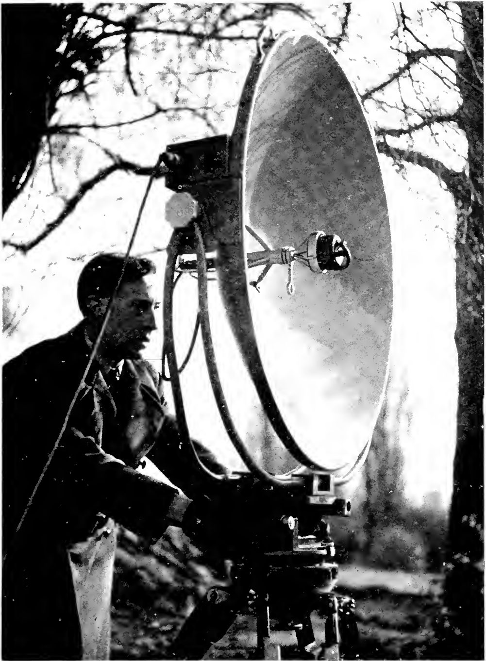
A 36-INCH PARABOLIC REFLECTOR OPERATED BY ERIC SIMMS. (Photograph by courtesy of THE B.B.C.).
