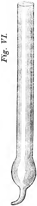
Glass tube for introducing blood into the living heart of a turtle (reduced one-half).
