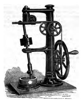
The machine consists of an iron pillar, two feet high, secured to a wooden base sixteen inches by twelve. The mortar rests in a ring on this base, and from the pillar, about half way up, extends an arm, at the end of which is a ball and socket, forming a sort of universal
