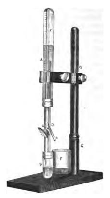
In using the apparatus 5 c.c. of the urine to be tested are put into the tube B, and A is filled with a solution of hypobromite of soda; on opening the stopcock the contents of A descend and give rise to a brisk effervescence in B. The gases evolved rise through the tube D, and are collected in A. The superfluous hypobromite solution flows into the beaker, F, and may be used again. When effervescence has nearly ceased the operation is completed
