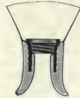
The Patent Constructed Neck (No. 118022) shows the brass socket embedded in rubber, rendering it impossible for water leakage to occur.
