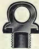
The Patent Rubber Covered Screw Stopper, No. 107940, in section.
