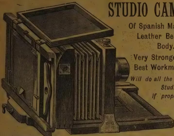
**THIS CAMERA** is perhaps the most useful Studio Camera extant. It has bellows body, extending in front by sliding and at back by endless screw, so that it has sufficient range to allow of its being used for the longest or shortest focus lens, and it may be used also for copying. It has swinging back, and takes the size plates quoted either way, horizontal or vertical. The ground-glass frame may either be hinged (as illustrated) or slide along when the dark slide is put in position.
