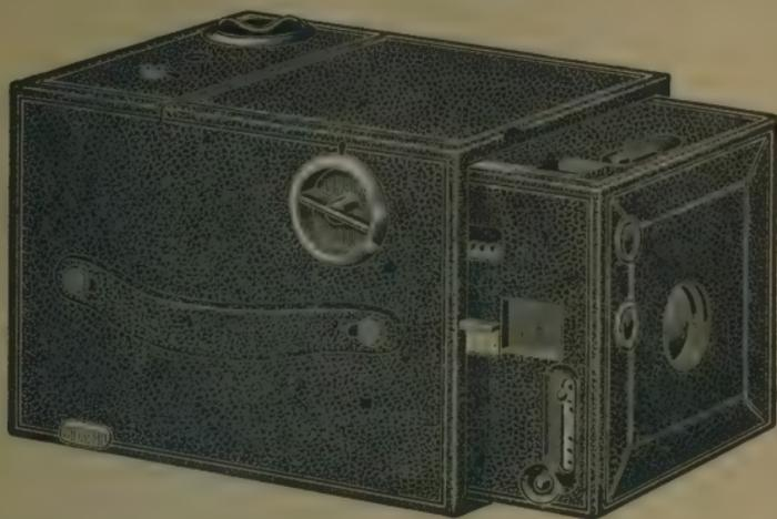
The model of this camera affords great compactness and quicker adjustment for use than the folding cameras. To focus, the inside case is projected by turning the sunken key, and the finders are located close to the scales.
