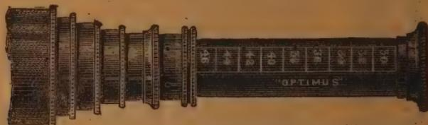
This diagram displays the Panratic Eye-piece. The figures represent magnifying power in diameters, which may be squared to ascertain number of times the object observed is amplified, thus  $46 \times 46 = 2116$  so that one superficial inch would appear enlarged that number of times.
