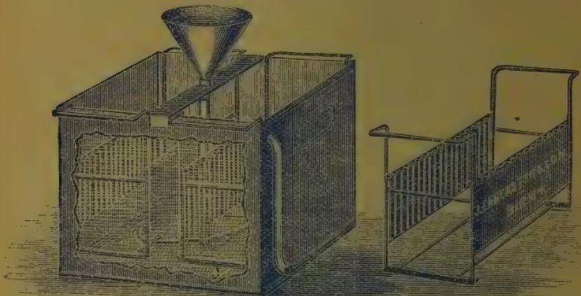
The "Hiero" Washer consists of a square metal vessel, japanned outside and enamelled white inside. It has two racks to hold the plates which may be used as dryers. The water enters through funnel and passes down centre tube and out of the bent ends, thus causing the funnel and tubes to rotate; this gives a supply of water under the whole of the plates, and keeps up a continuous circulation, the waste being emptied periodically by the Syphon on side.
