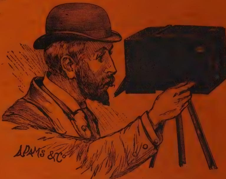
Fig. 141A.—Showing Camera used on a Tripod, with object being focussed upon the focussing screen; also showing rising front and swing back in use.
