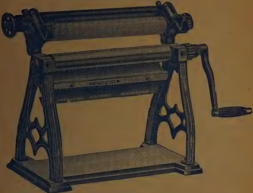
THIS machine is superior to any other Rotary Burnisher ever offered to the Photographic fraternity. This Burnisher has our patented one wheel end adjustment which is the most perfect device ever applied to a Burnisher for securing uniform pressure and giving perfect accuracy of adjustment with one motion; also, our patented device for maintaining uniform pressure.
