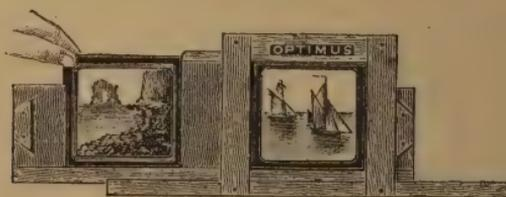
or less complicated description. The patent represented in the diagram is exceptional, from the fact that it has neither levers nor springs nor mechanical confusion of any kind whatsoever. Its individuality and efficiency are nevertheless very pronounced. The movement of the lantern photographs is obtained by the usual sliding action, whilst the absence of the top bar of the inner frame permits the fingers to freely withdraw the exposed and insert the fresh transparency.
