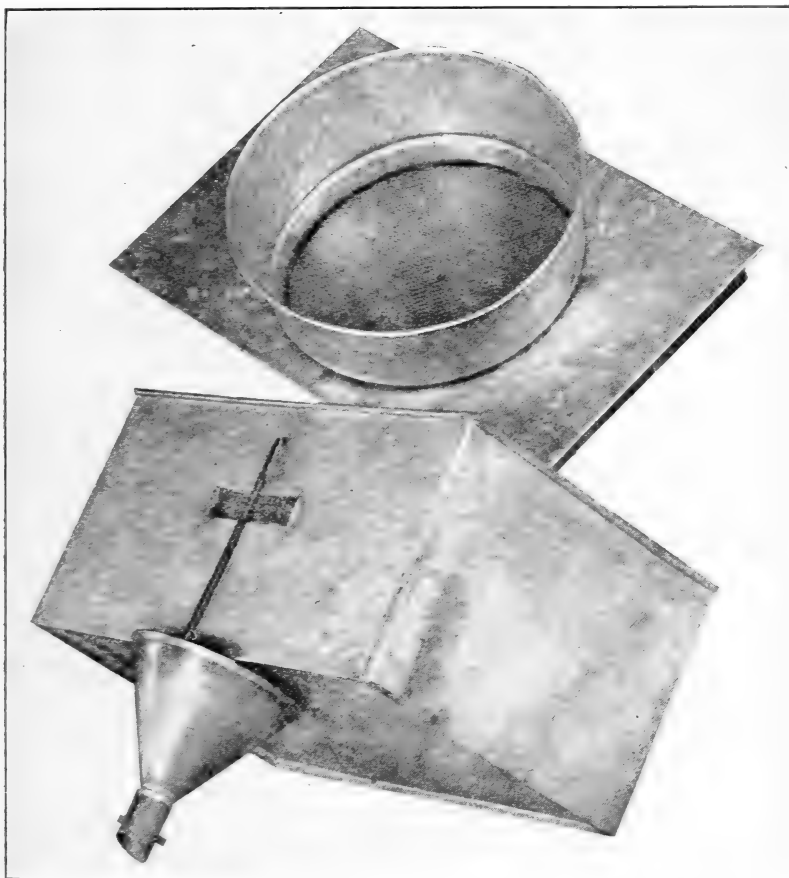
FIG. 14.—Automatic oil-measuring device
