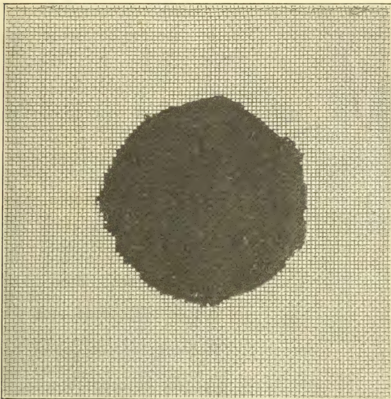
FIG. 12.—Wire gauze, with asbestos center
