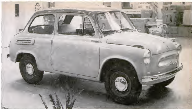
Vents above rear wheels supply air for cooling ZAZ engine. The car's top speed is 55 m.p.h.
