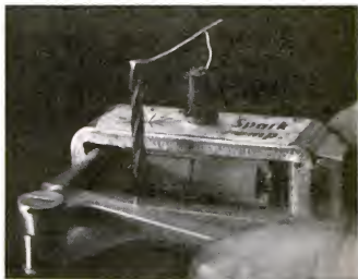
SQUEEZING A LEVER rigged to work this piezoelectric spark pump creates a half-inch flash of electricity. The ceramic is compressed only slightly—1½ thousandths of an inch.
