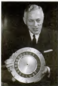
TURBINE ENTHUSIAST Huebner holds variable nozzle plate for power turbine. It has 23 vanes that can rotate, automatically, 100 degrees.
