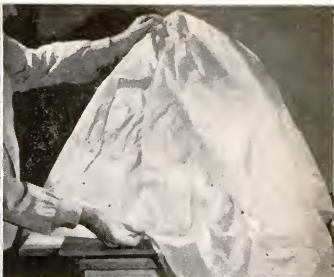
AFTER ADDING BARREL to dome, attach the first of the four cone segments. They are seamed to bottom edge of barrel one at a time, then joined to each other. These are trickiest seams.
