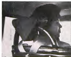
WEBBED STRAPS behind rear-seat passengers' heads prevent whiplash injury, and armrest stops sliding during a lateral collision. Belts and harnesses give added protection.
