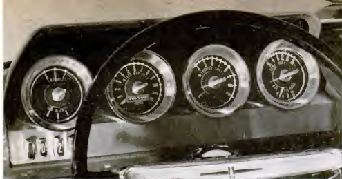
INSTRUMENTS , left to right: (1) amps, fuel gauge; (2) speedometer; (3) turbine speed as percentage of maximum, graduated in tens; (4) turbine inlet temperature in hundreds, oil pressure in tens. Accelerator governs fuel-pump r.p.m. Problem is turbine blade's low heat tolerance. Goal: 2,000 degrees—80 more hp.
