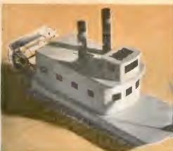
Sun boat: Solar power turns its paddles. P. 119
