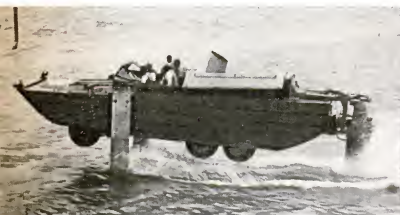
FLYING DUCK , foilborne amphibian vehicle with wheels, was tried out last year by U. S. Army. The 13-ton craft, with submerged foils and gas turbine, skims the water at 35 m.p.h.
