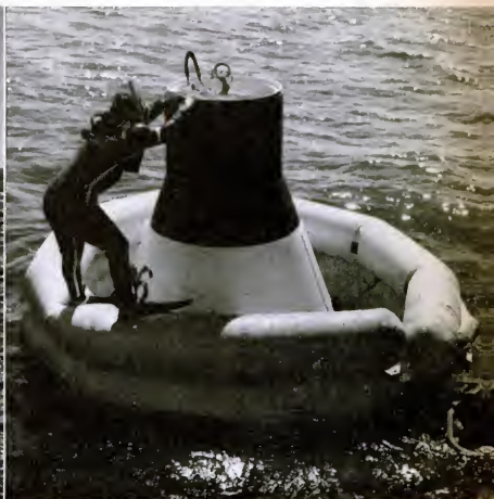
DUMMY SPACE CAPSULE —a steel mockup of the one used by Mercury astronauts—is here used by the par divers as a rescue problem in their training program. Big inflated collar they have just fastened around the capsule was adapted from a standard GI 20-man lift raft.
