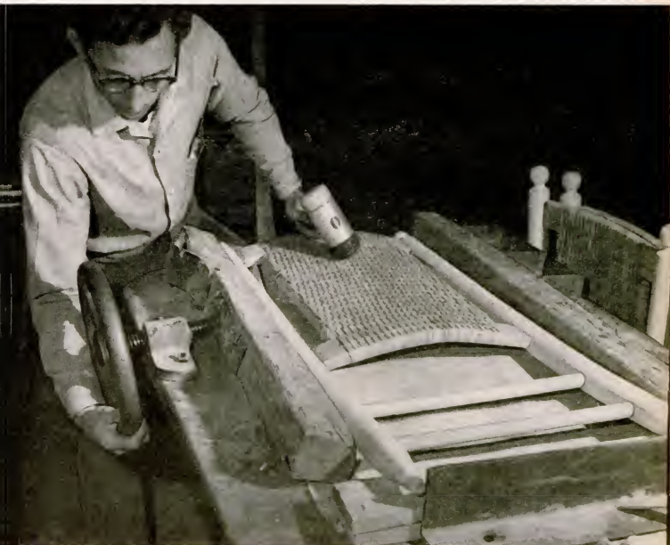
9. ASSEMBLY LINE GOES INTO ACTION whenever a supply of seats and back rests comes down from the weavers. This horizontal screw press forces posts onto back rest and rungs, while
