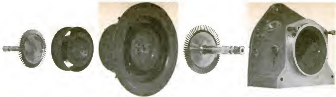
EXPLODED VIEW shows accessory case (oil, fuel, air pumps) at far left; compressor, turbine
