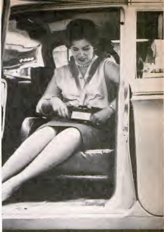
CAPSULE CHAIRS swivel 360 degrees for easy entry and exit. The flick of a single buckle latch instantaneously releases the lightweight lap belt and both shoulder straps.
