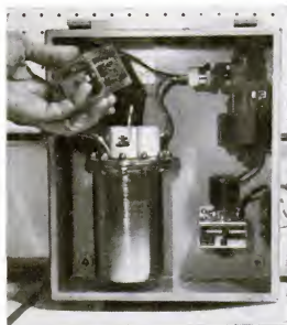
MINIATURIZATION shrinks newer model to half size. Hand is holding electronic brain that translates signals from flow and temperature sensors to control current from the rectifier.
