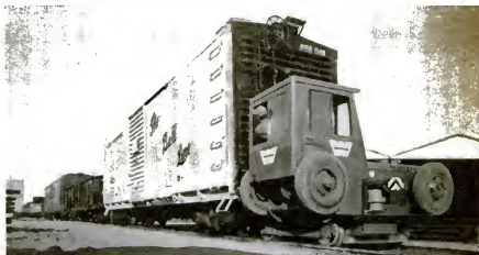
Truck wheels up and riding sideways, it's a switch engine.
