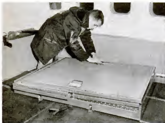
Folded container bolts to floor of plane cabin.
