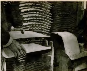
6. SIMPLE SETUP above resembles a pencil sharpener in its operation. Square end of band-sawed armrest is placed in a guide and pressed into a spinning cutter head that rounds and tapers it to fit hole bored in rear post.
