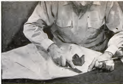
JOIN DOME HALVES after putting gores together in fours. Use the same type of seam, pressing with a putty knife to keep edge of top piece flat while bottom one is folded up over it.
