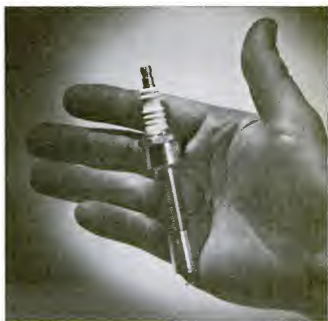
SINGLE SPARK PLUG is five inches long to extend into burner. Burner cap, which carries it, supplies both air and fuel to the burner. Extra compressor air is vital to turbine speed.
