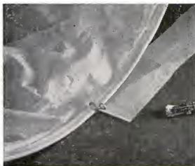
PASTE RING INSIDE MOUTH and reinforce seam with paper strip folded over it and lapped \frac{1}{2} " over each side of balloon tissue. Before applying, attach hooks at 120-degree points.
