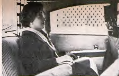
WEBBED STRAPS behind rear-seat passengers' heads prevent whiplash injury, and armrest stops sliding during a lateral collision. Belts and harnesses give added protection.
