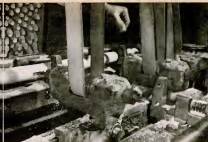
5. MORTISING MACHINE can rout up to three mortises simultaneously. Here two router heads oscillate rapidly from side to side on a carriage, while the operator feeds the post toward them until the required depth is reached.
