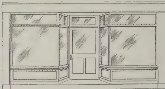
Fig.—Front Elevation of Show Windows
