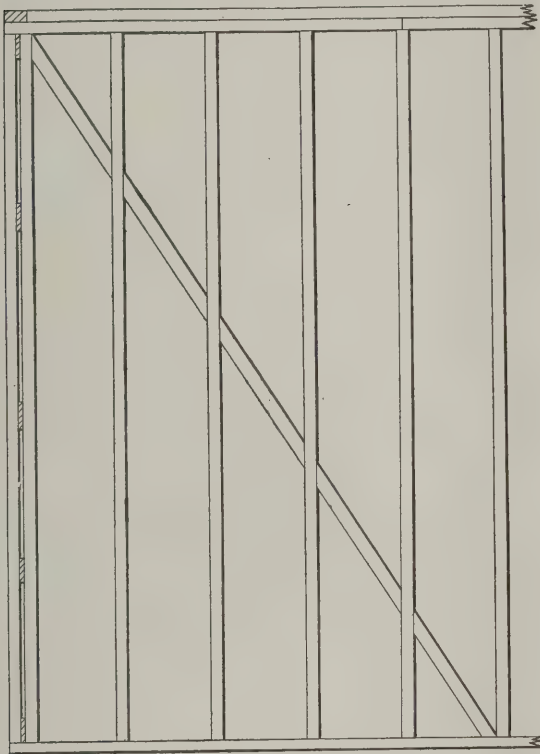
Fig. 1—Style of Bracing Used in Balloon Framing.
