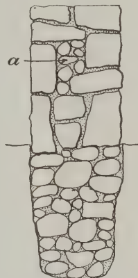
Fig. 5—Incorrect Method of Building a Wall on a Trench Foundation.
