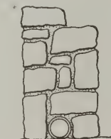
Fig. 2—Incorrect Location of Tile Drain.
