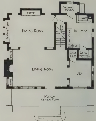
Main Floor—Scale 1/16 In. to the Foot
