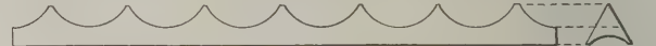
Fig. 212.—Enlarged View of Cresting on Top Rail of Fence Shown in Previous Figure—Scale 1\frac{1}{2} in. to the Foot.
