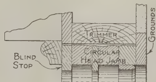
Section of Head on Line D-D of the Elevations—Scale 1 1/2 In. to the Foot
