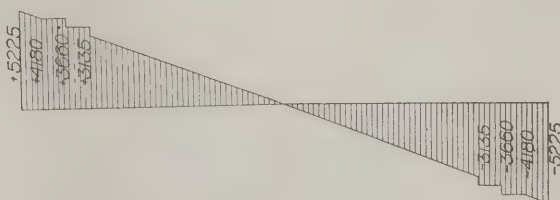
Fig. 50—Shear Diagram for a Reinforced Beam
