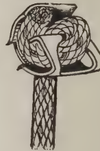
Fig. 14—The Fastener Applied to Sash Cord
