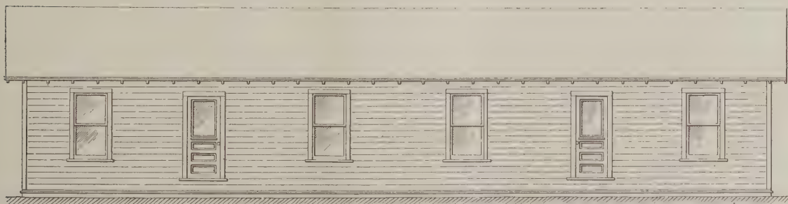
Front Elevation Showing Position of Windows and Doors.—Scale \frac{3}{32} In. to the Foot
