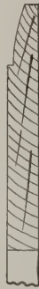
Continuous Trim in Living and Dining Rooms and Reception Hall—Scale 3 In. to the Foot
