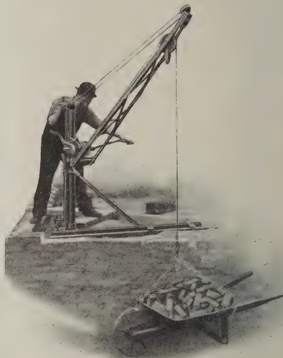
Fig. 7—An All-Steel Builder's Derrick
