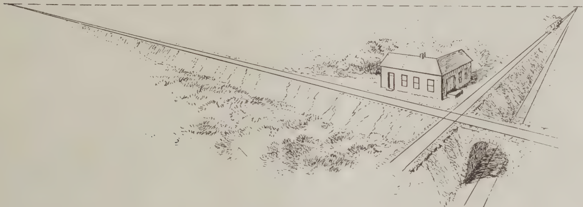
Elementary Perspective Drawing—Fig. 2—Finding Vanishing Points by Observation on Two Railroads Crossing Each Other
