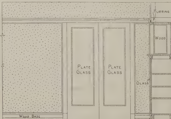
Elevation of Doors from Living Room to Porch with Section Through Bookcase—Scale 1/4 In. to the Foot
