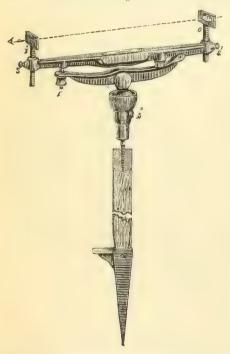
struction. To make its operations perfectly plain, the following example is given:—Problem.—To set a number of stakes or pegs in the ground, to define the surface of a proposed concrete floor for instance, so that their top ends shall be in the same horizontal plane—and at the same time so that all the pegs shall be of the same level as some other peg, marked
