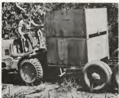
Loading bins on a low-bed trailer.
