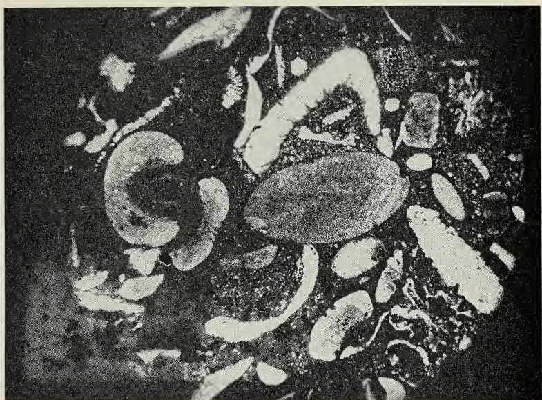
Figure 12 Microphotographs. Left, oölitic hematite with nuclei of quartz in groundmass of hematite and calcite, x 80; right, red flux showing hematite (dark) and calcite (light) in bryozoans and groundmass, x 80.
