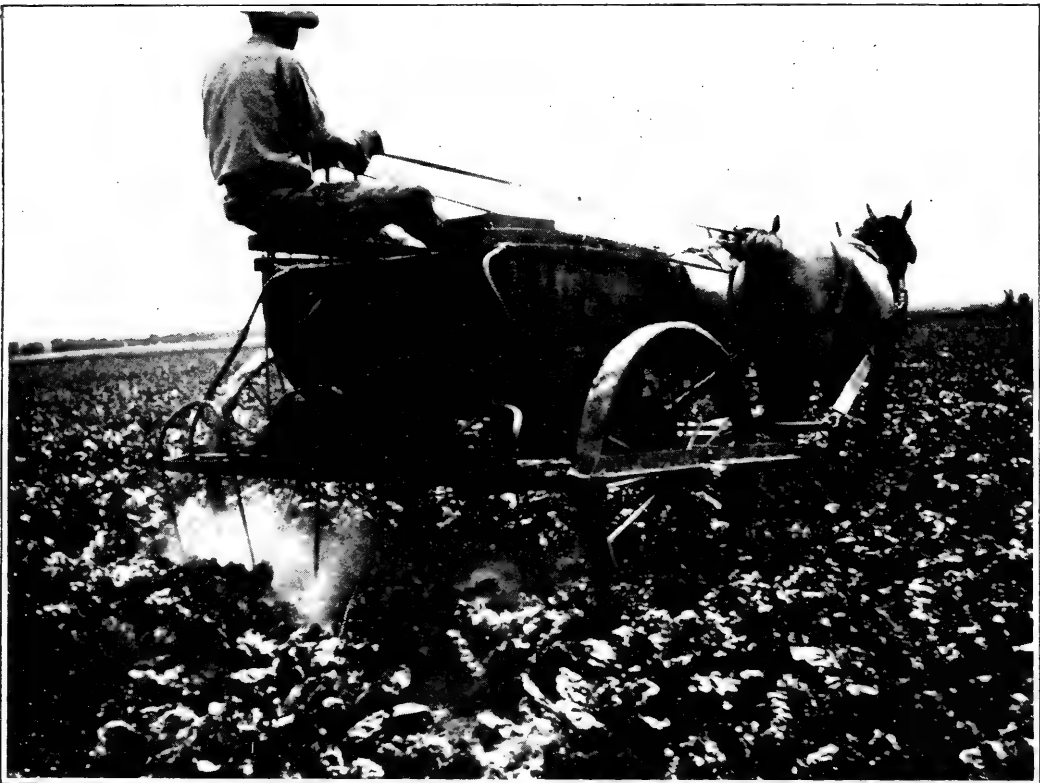
FIG. 2.—GEARED TRACTION SPRAYER IN OPERATION IN SUGAR-BEET FIELD AGAINST THE HAWAIIAN BEET WEBWORM. (ORIGINAL.)
