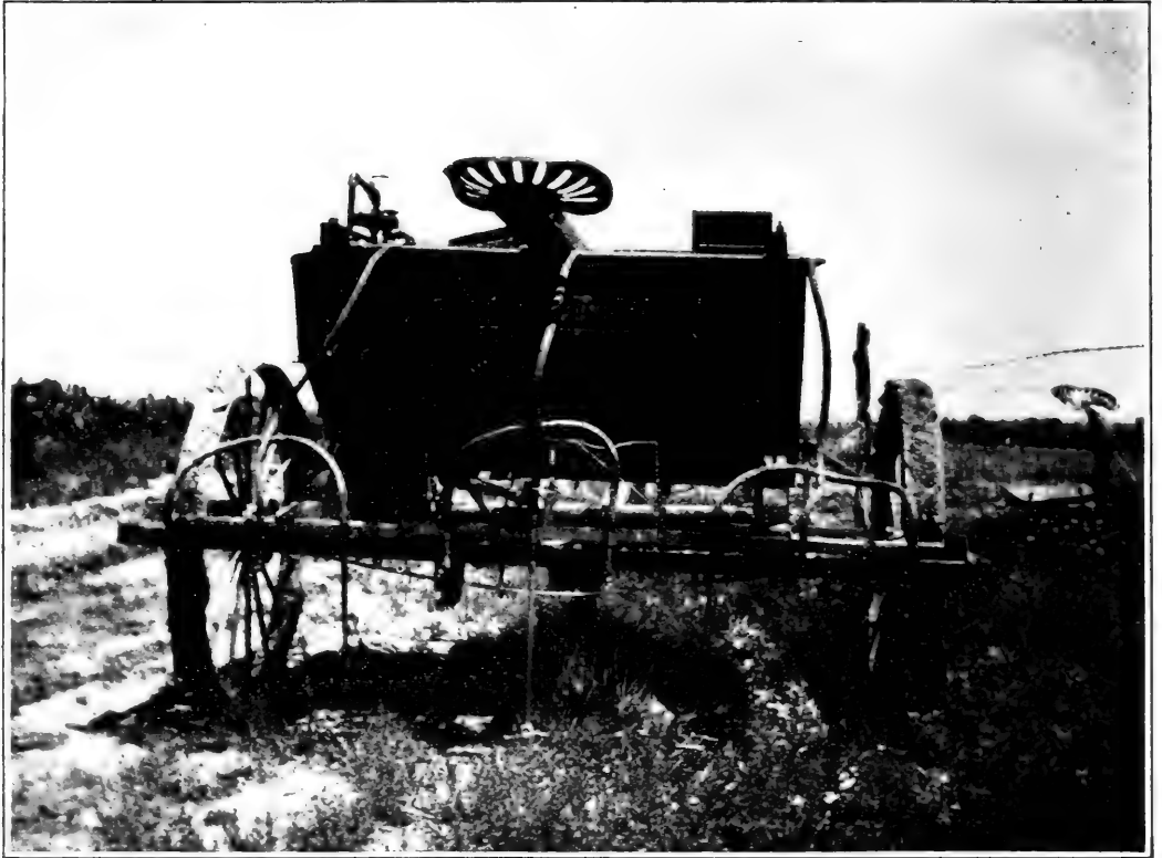
FIG. 20.—Geared traction sprayer suitable for use against the sugar-beet webworm. (Author's illustration.)
