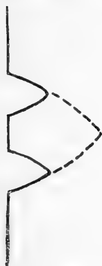
FIGURE 3.—Manner of cutting tree preparatory to felling.
