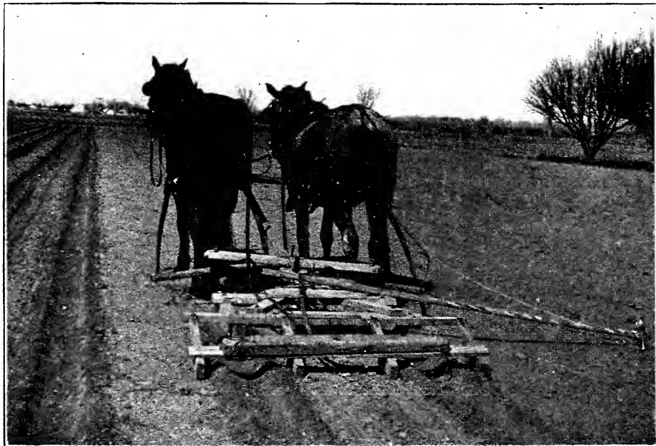
No. 11.—A marking and logging out device for seeding and irrigating alfalfa in rows, to prevent surface flooding of the soil.
