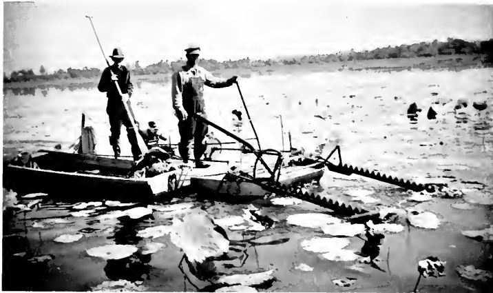
Fig. 32.—Machine for mowing aquatic plants. At the Lake Chautauqua National Wildlife Refuge, where this machine is shown in operation, it was possible to mow an acre of American lotus per hour.
