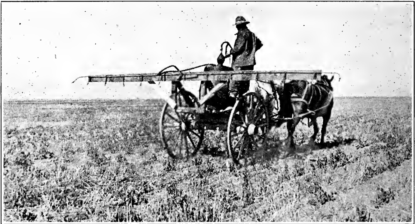
Fig. 7.—A 13-nozzle beet spraying machine. The type that was used in the grasshopper campaign, 1916, San Luis Valley. (Original).
