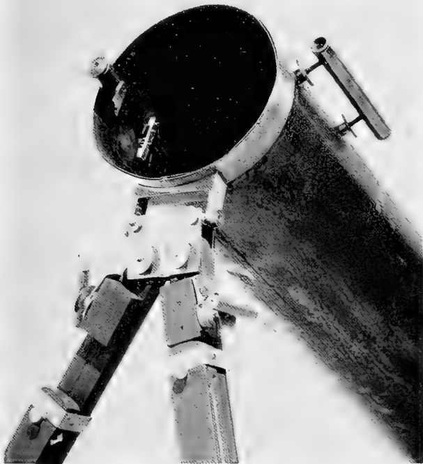
FIGURE 3.—Eyepiece and tripod head of the Holcomb reflecting telescope shown in figure 2. (Smithsonian photo 11000)
