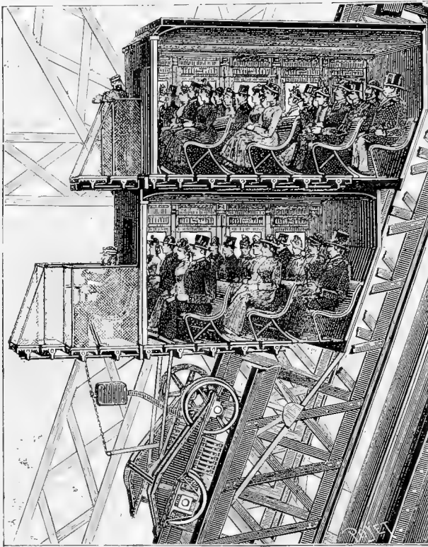
Figure 29.—Section through cabin of the Otis elevator. Note the pivoted floor-sections. As the car traveled, these floor-sections were leveled by the operator to compensate for the change of inclination; however, they were soon removed because they interfered with the loading and unloading of passengers. (From La Nature , May 4, 1889, vol. 17, p. 360.)
