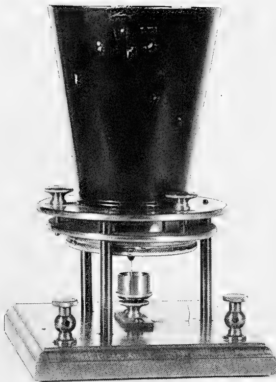
FIGURE 63.—Reproduction of Bell's liquid transmitter, his first successful instrument to transmit articulate speech (March 10, 1876). (USNM 252600; Smithsonian photo 47876.)
