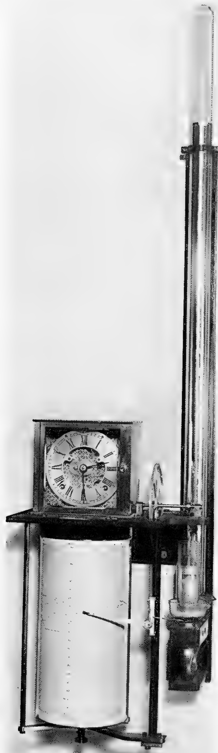
Figure 14.—Marvin's mechanical registering barometer, 1905. This instrument was formerly in the U.S. Weather Bureau. (USNM 316500; Smithsonian photo 46740-E.)
