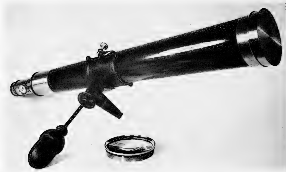
FIGURE 9.—Refracting telescope, comet seeker, (USNM 317027) by Henry Fitz, 8\frac{1}{4} -inch aperture, 61-inch tube, fitted for equatorial mounting. The stand is lacking. ( Smithsonian photo 46815 )
