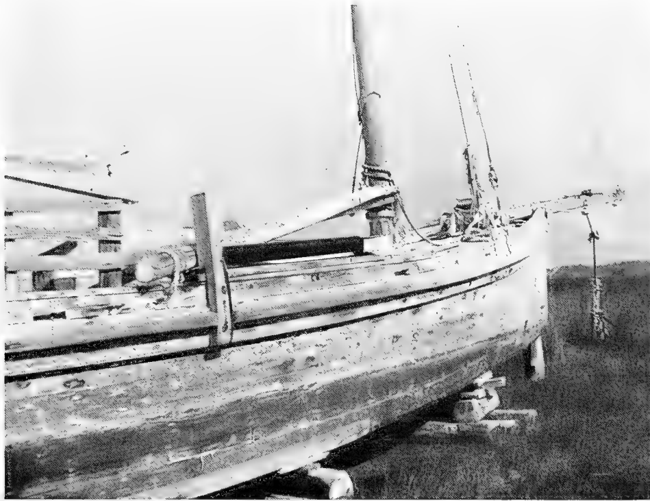
FIGURE 14.—The entrance of a North Carolina sharpie schooner and details of her sharp lines and planking. Note scarphs in plank.
