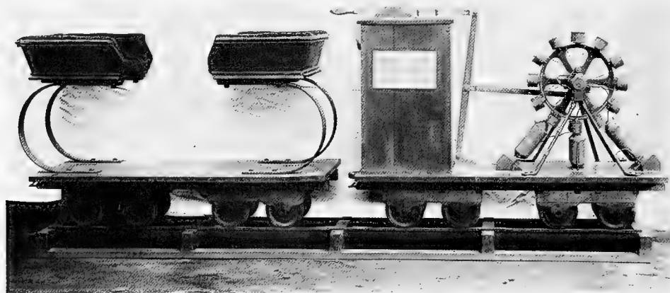
Figure 70.—Reproduction model of Farmer's electric train. The locomotive is about 4 feet in length. ( USNM 181348; Smithsonian photo 14588. )
