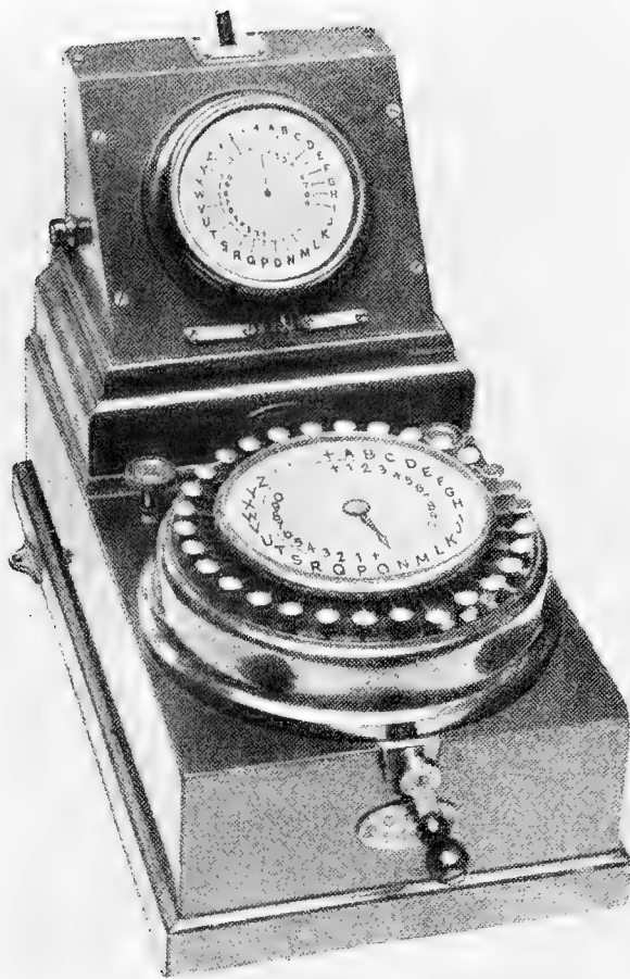
FIGURE 25.—Wheatstone's ABC telegraph, an instrument made in 1876 and based upon the patent of 1860. From E. Feyerabend, Der Telegraph von Gauss und Weber , Berlin, 1933, p. 79.
