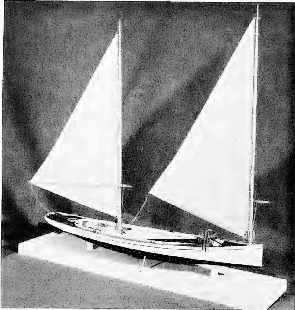
FIGURE 1.—Scale model of a New Haven sharpie of 1885, complete with tongs. (USNM 318023; Smithsonian photo 47033-C.)
