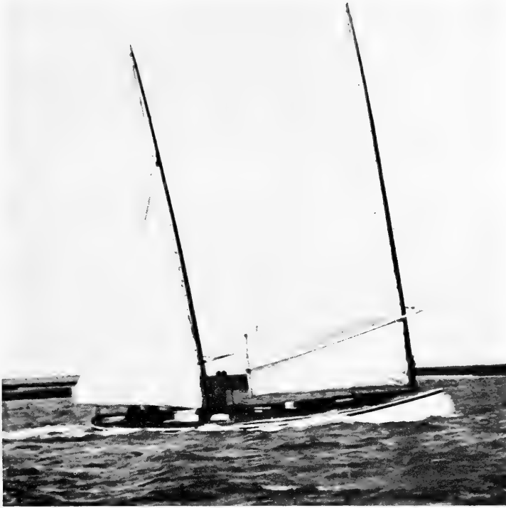
FIGURE 6.—North Carolina sharpie with one reef in moderate gale, about 1885. (Photo courtesy Wirth Munroe.)
