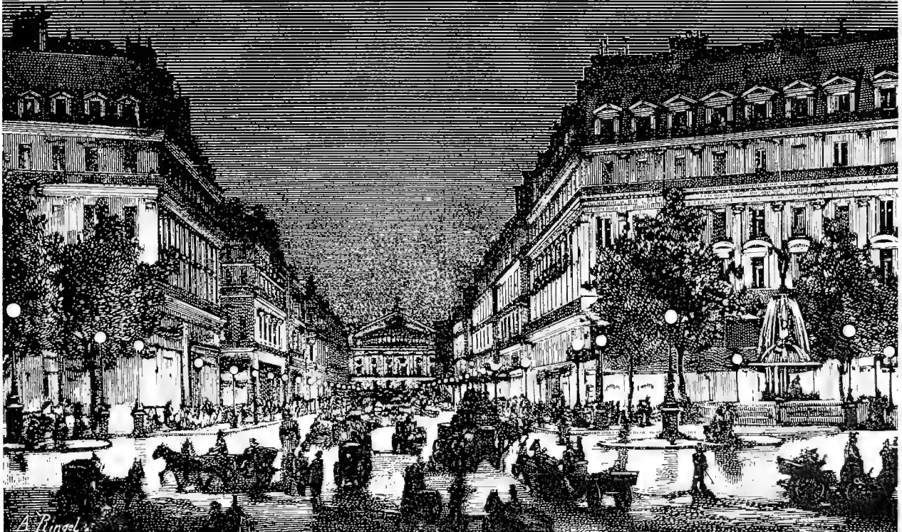
Figure 84.—Avenue de l'Opéra in Paris as illuminated by Jablochhoff candles in 1878. From La Lumière électrique , 1881, vol. 4, p. 186.
