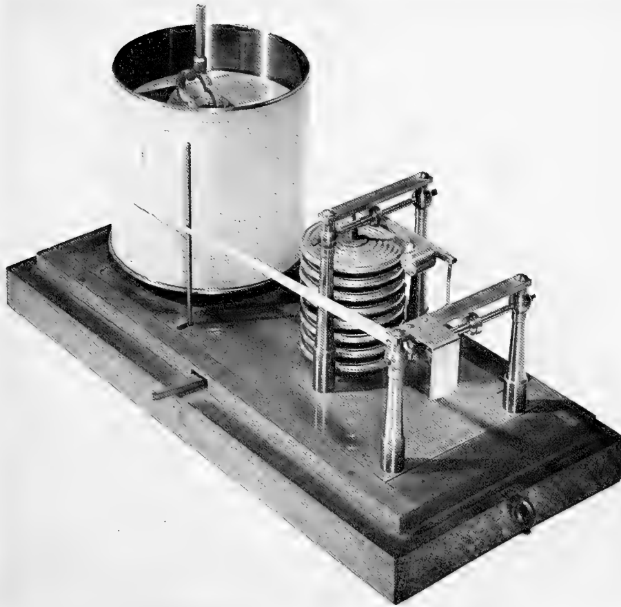
Figure 16.—Richard's registering aneroid barometer, an instrument used at the U.S. Weather Bureau about 1888. The Richard registering thermometer is similar, the aneroid being replaced by an alcohol-filled Bourdon tube. ( USNM 252981; Smithsonian photo 46740-C. )
