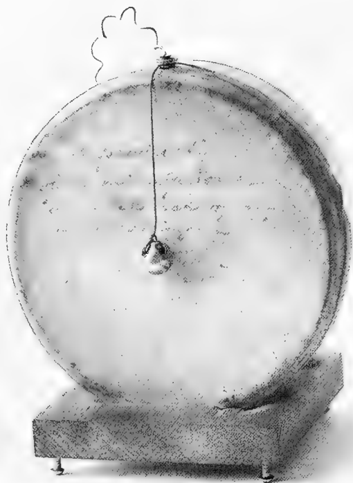
FIGURE 70.—Reproduction of Berliner's toy drum microphone. The contact was a needle that pierced a drum membrane against which a metal ball rested. (USNM 309377; Smithsonian photo 42367.)
