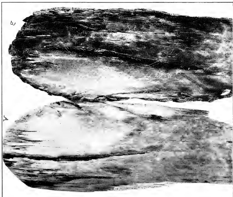
FIG. 2.—EVIDENCE OF CUTTING OF LIVING TREES. A, SCORING CHIP FROM RAILROAD TIE, SHOWING SURFACE OF WOOD NOT MARKED BY INSECTS; B, INNER SURFACE OF BARK FROM SAME CHIP, ABOUT ONE-THIRD NATURAL SIZE. (ORIGINAL.)
