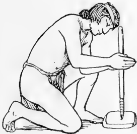
FIG. 216. Primitive method of drilling.
