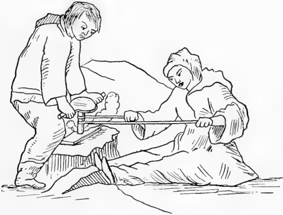
FIG. 220. Primitive method of drilling.
