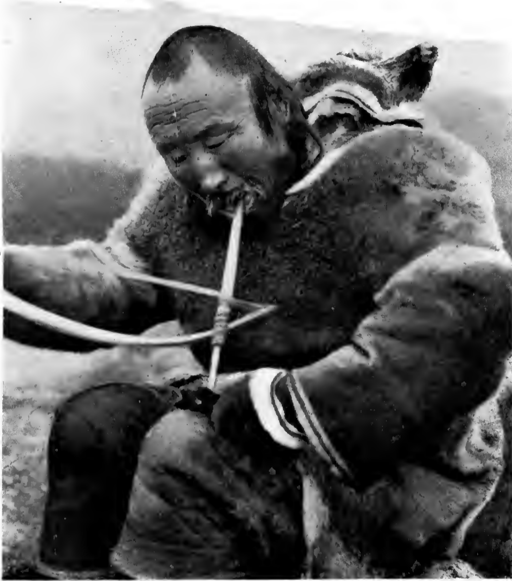
An Eskimo of the Mackenzie River delta using a bow-drill for piercing bone. ( Photo by J. R. Cox. )
