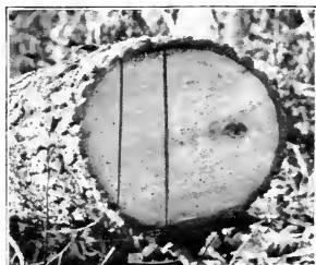
FIG. 18.—Cross section of a fallen Black Oak. Milford, Pa. The slabs shown in figs. 19 and 22 were sawed lengthwise from this tree, beginning where the black lines are seen on the cross section.
