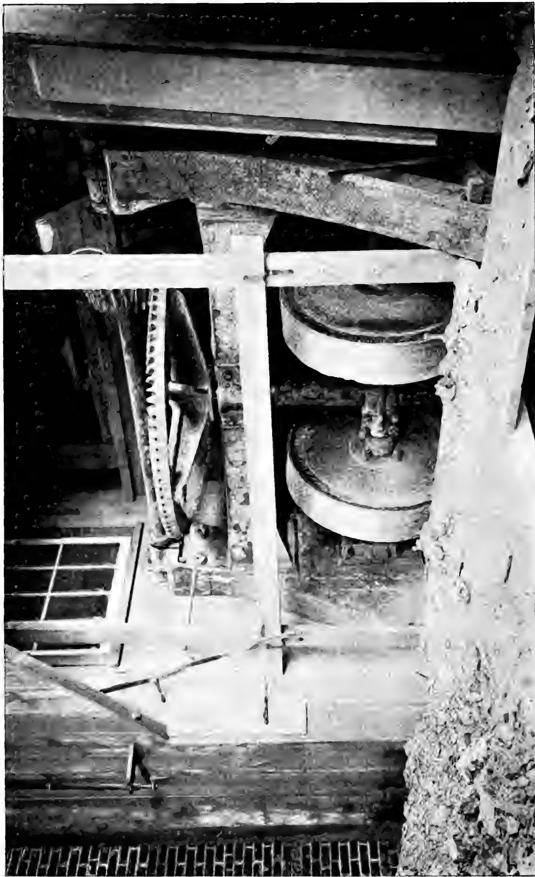
Dry pan for grinding shale, Celadon terra cotta co., Alfred Center.
