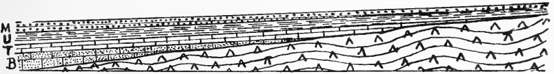
Fig. 13 Diagram to illustrate the condition of the region after deposition of the Paleozoic rocks and emergence above sea level, with smooth, southerly sloping surface B=Beekmantown, T=Trenton, U=Utica and Hudson shales and M=the Oswego and Medina sandstone formations of the Upper Silurian.
