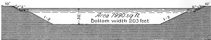
Fig. 58 Earth section of deep waterways for 30-foot channel.
