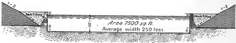
Fig. 57 Cross-section of deep waterways, partly in rock and partly in earth, for 30-foot channel.
