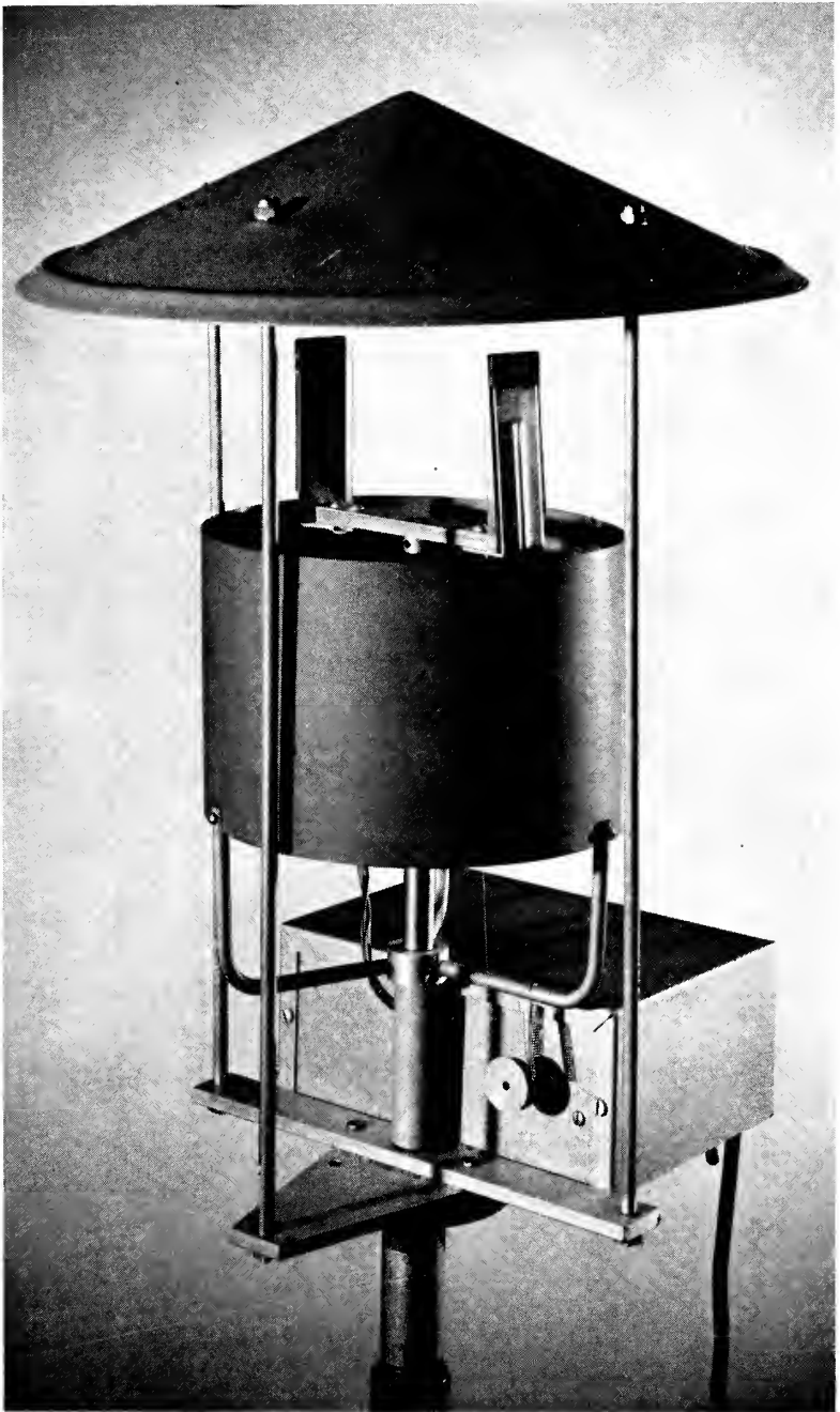
Figure 4. The intermittent rotoslide pollen sampler is widely used for obtaining the pollen count and for research in aerobiology.
