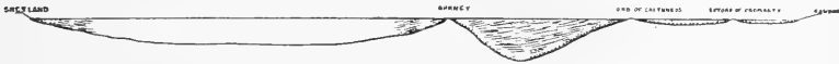
FIG. 18. SECTION TO EXPLAIN THE DEPOSITION OF THE OLD RED SANDSTONE IN THE NORTH OF SCOTLAND (After Geikie)
