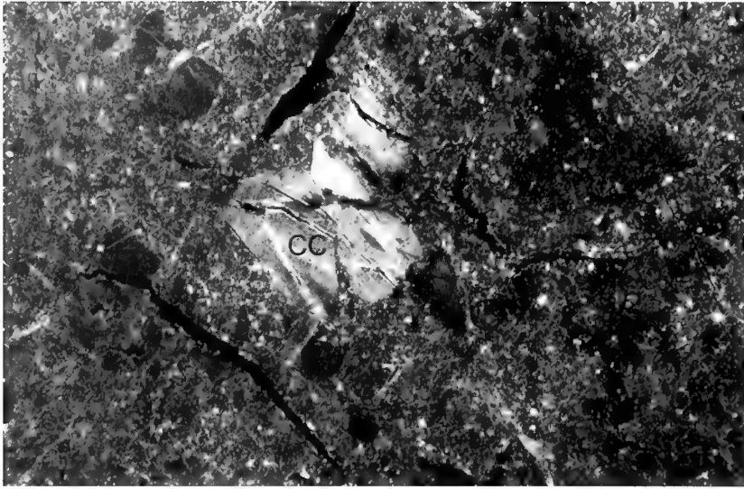
Fig. 5 Sample C from the sand hole, a basal clay deposit including a locally reworked clay (CC). Note the reticulate birefringent fabric which is indicative of minor shrinking and swelling reflecting alternate periods of wetting and drying. Width of photo ca. 5.4 mm.
