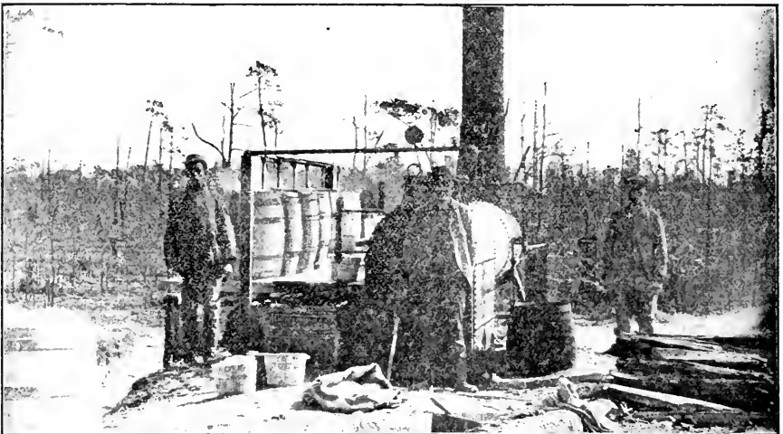
Fig. 5.—Steam-boiler outfit for making Lime-sulphur Wash for orchard of 35,000 peach trees. Moore County, N. C. (Photo by Sherman.)
