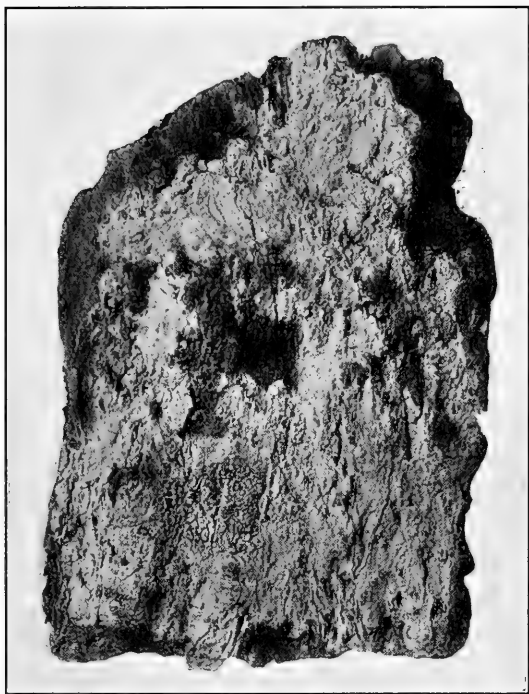
FIG. 1. EVANSITE COATING COAL. WHITE, EVANSITE; BLACK, COAL. NOTE BOTRYOIDAL CLUSTERS BELOW THE BLACK SQUARE IN CENTRE.
