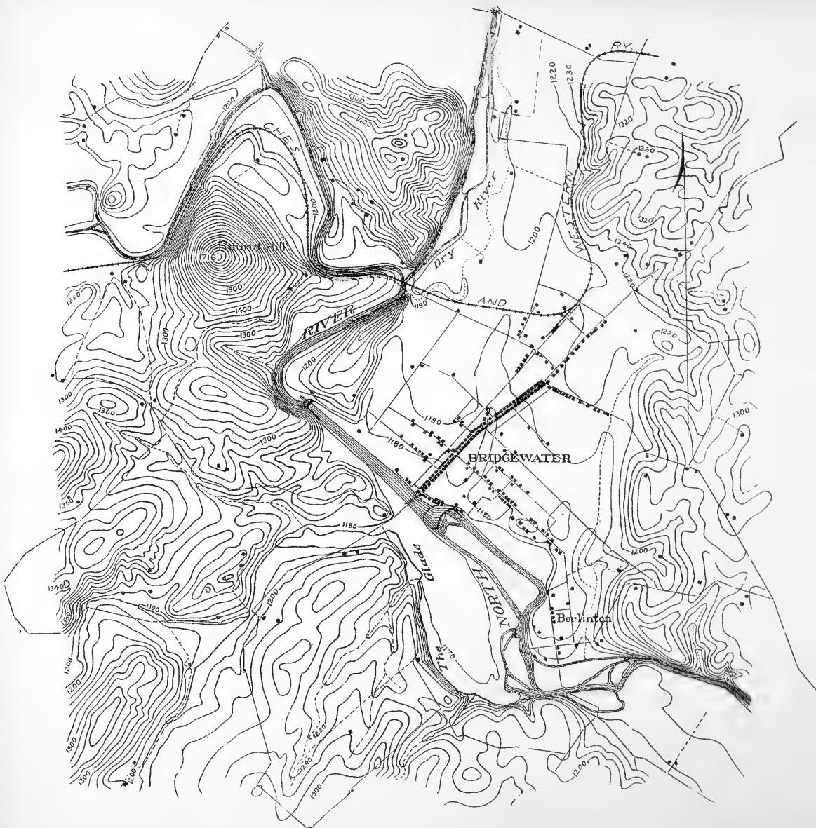
FIG. 4. TOPOGRAPHIC MAP OF BRIDGEWATER AND VICINITY, ROCKINGHAM COUNTY, VIRGINIA. Scale 2.667 inches = 1 mile. Contour intervals 10 and 20 feet.
