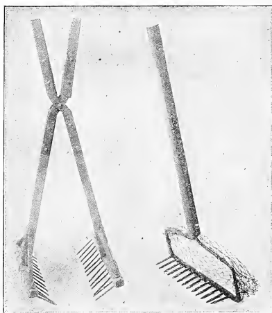
Tongs and rake used in mussel fishery of Mississippi River.
