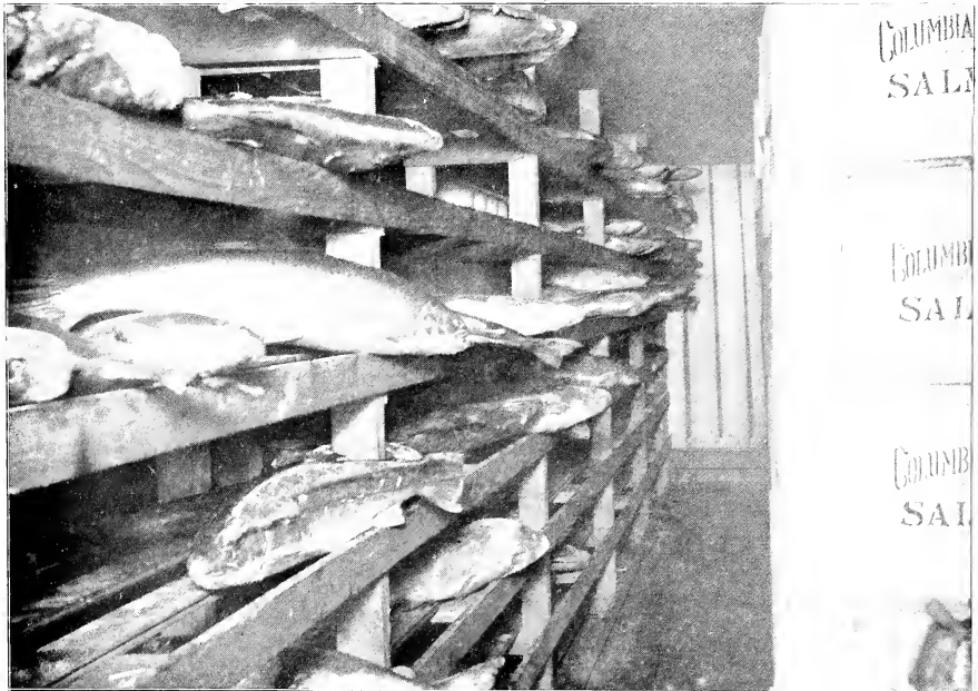
INTERIOR OF ICE-AND-SALT FREEZING-ROOM ON PACIFIC COAST, CONTAINING SALMON AND STURGEON. (See page 582.)
