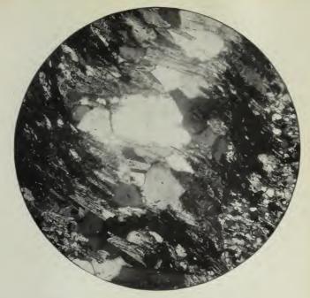
A. MICACEOUS AND QUARTZOSE SCHIST WITH CLEAVAGE ACROSS BEDDING.
