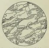
FIG. 18.—Feldspar in perallel lenses with crystallographic parallelism. The longer axes of the lenses are approximately in the brachypinacoid. From hornblendic schist of Mesabi district of Minnesota.
