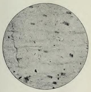
B. SLATE WITH FALSE CLEAVAGE.
