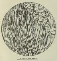
FIG. 34.—Fracture cleavage in slate emphasized by ferruginous staining. There are 360 cleavage planes to the inch. After Dale.
