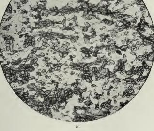
HORNBLENDIC SCHISTS. Showing arrangement of hornblende cleavage in slides cut across the schistosity.
