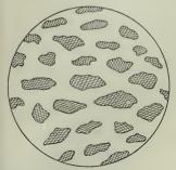
FIG. 6.—Sketch showing tendency toward parallelism of dimensional axes and cleavage of hornblende as viewed in basal section.
