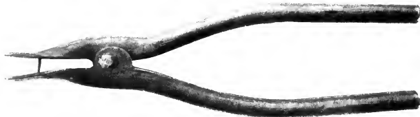
FIG. 2.—A tool which, if employed with care, may be used for partially opening living mussels for examination of conditions within the shell.
