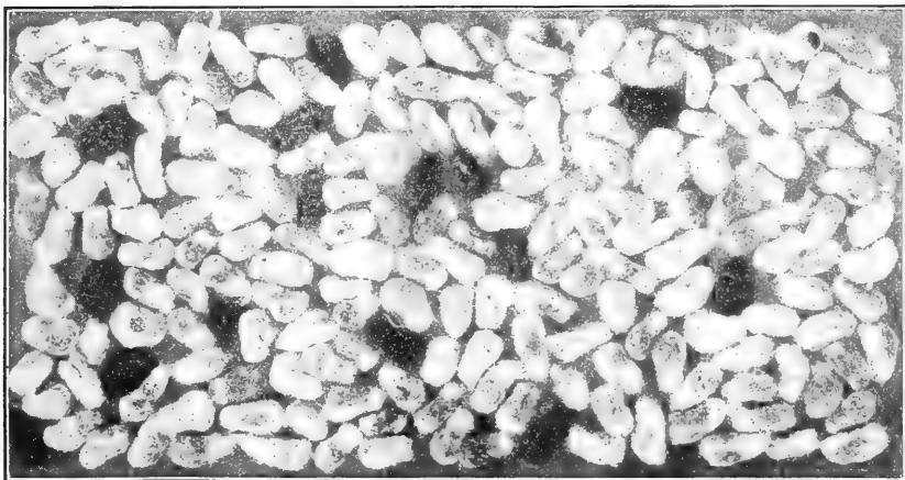
FIG. 3.—Sample of cotton seed taken 15 minutes after the ginning of the second bale had begun, showing 7.4 per cent of red seed from the stained roll of the first bale.
