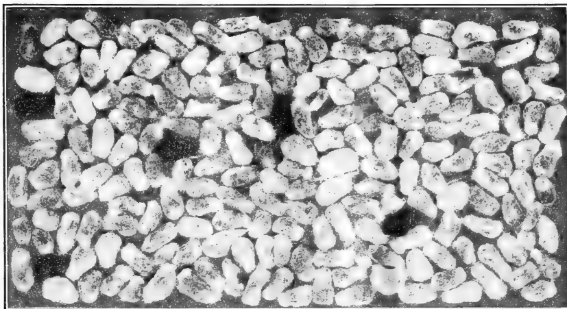
FIG. 4.—Sample of cotton seed taken 20 minutes after the ginning of the second bale had begun, showing 2.8 per cent of red seed from the stained roll of the first bale.
