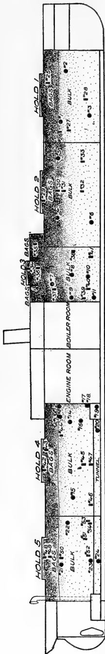
Fig. 35.—Diagram showing arrangement of the steamship and stowage of the corn in holds. The heavy shading represents heat-damaged corn as discharged. (Cargo No. 5.)
