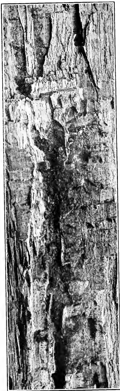
DAMAGE TO SOLID OAK WOOD BY RETICULITERMES HUMILIS , VAR. HOFERI IN ARIZONA.
