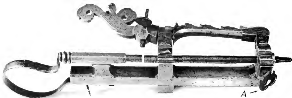
Figure 3. SMALL THREAD-CUTTING LATHE which was made to be held in a vise during use. It was found as shown here, with only the operating crank missing. The overall length is approximately 12 inches, depending on the adjustment of parts. (Smithsonian photo 16525B.)
