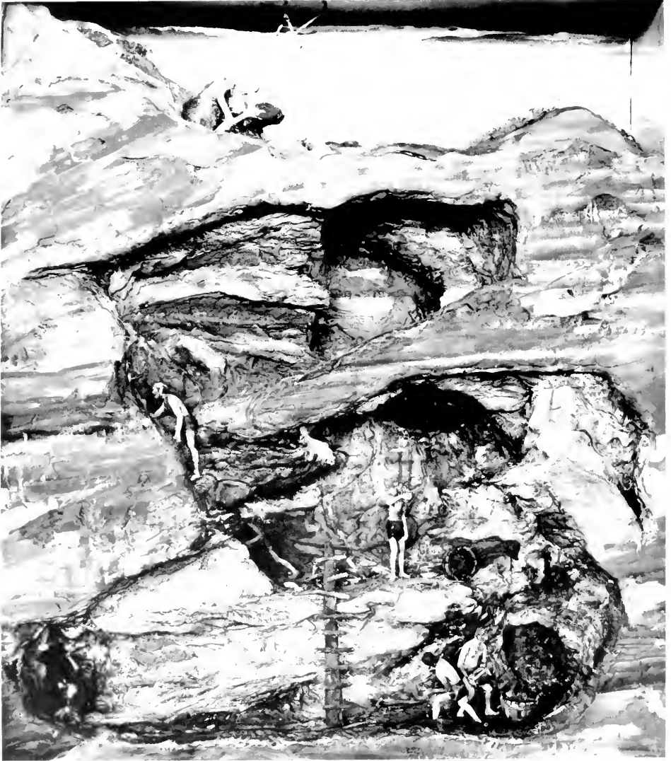
FIGURE 1. MINING BY EARLY EUROPEAN CIVILIZATIONS, using fire setting and hand chiseling to break out ore and rock. MITI model, \frac{1}{4} " scale. (Smithsonian photo 49260, H.)
