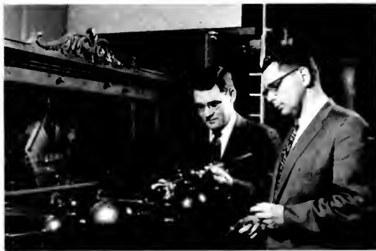
Figure 19.—CURATORS JOHN B. BLAKE AND GEORGE GRIFFENHAGEN examine the newly acquired (1957) electromagnetic, Morton-Wimshurst Holz Influence Machine. It was manufactured by the Bowen Company of Providence, Rhode Island (1889). With the discovery of x-ray, it was used for making x-ray photographs until early in the 20th century.
