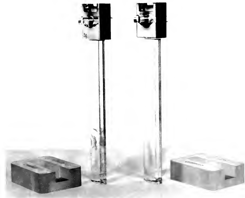
Figure 20.—THE GULF PENDULUM is about 10.7 inches long, and has a period of .89 second. It is made of fused quartz which is resistant to the influence of temperature change and to the earth's magnetism. Quartz pendulums are subject to the influence of electrostatic charge, and provision is made to counteract this through the presence of a radium salt in the case. The bearings are made of Pyrex glass.
