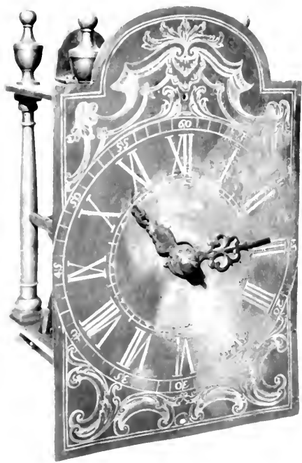
Figure 26.—DIAL PLATE of a brass lantern clock made by Bertolla, found in his workshop after his death. (Courtesy of Museo Nazionale della Scienza e della Tecnica, Milan.)
