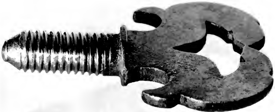
Figure 8.—BINDING SCREW seen at a in figure 3, showing the long smooth fadeout of the thread below the shoulder. (Smithsonian photo 40276.)
