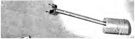
FIGURE 20.—PISTON AND CONNECTING ROD of second engine. Screw on rod is where oil is poured into connecting rod to lubricate wrist pin and crankshaft.
