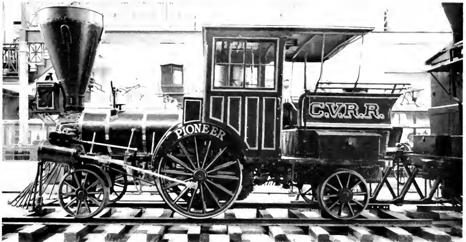
Figure 16. - The "Pioneer" as first exhibited in the Arts and Industries building of the Smithsonian Institution prior to restoration of the sandbox. (Smithsonian photo B060D.)
