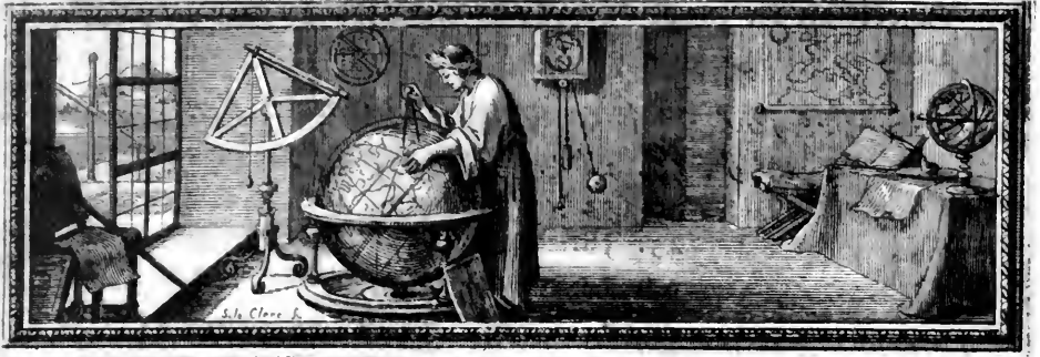
Figure 2.—THIS DRAWING, FROM RICHER'S Observations astronomiques et physiques faites en l'isle de Caienne (Paris, 1679), shows most of the astronomical instruments used by Richer, namely, one of the two pendulum clocks made by Thuret, the 20-foot and the 5-foot telescopes and the large quadrant. The figure may be intended as a portrait of Richer. This drawing was done by Sebastian Le Clerc, a young illustrator who made many illustrations of the early work of the Paris Academy.
