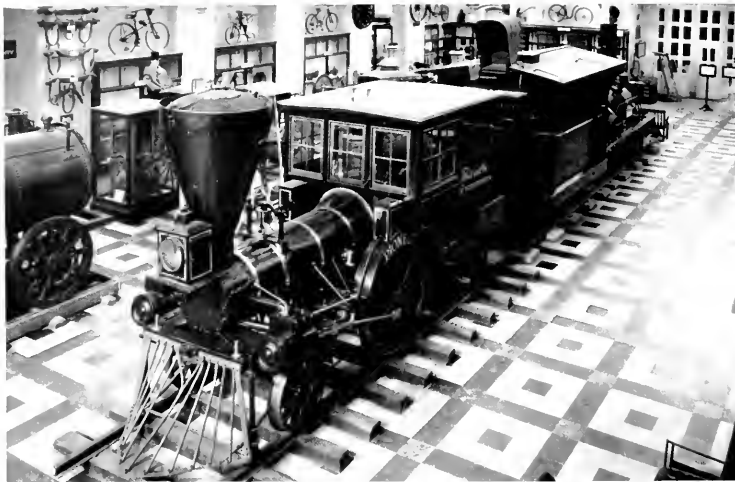
Figure 21.—“PIONEER” ON EXHIBIT in old Arts and Industries building of the Smithsonian Institution. In this view can be seen the bonnet screen of the stack and arrangement of the boiler-frame braces and other details not visible from the floor. (Smithsonian photo 48069A.)
