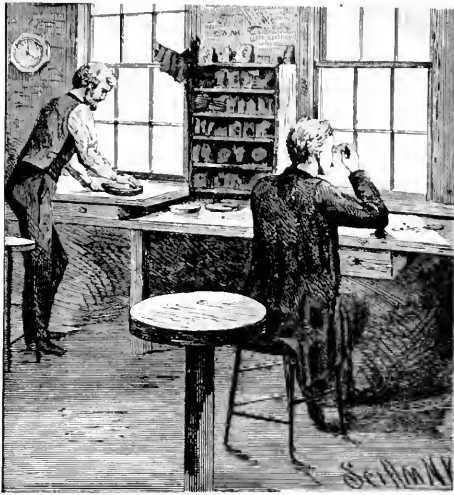
FIGURE 16.—Polishing lenses in the Alvan Clark & Sons factory. From cover of Scientific American , 24 September 1887.
