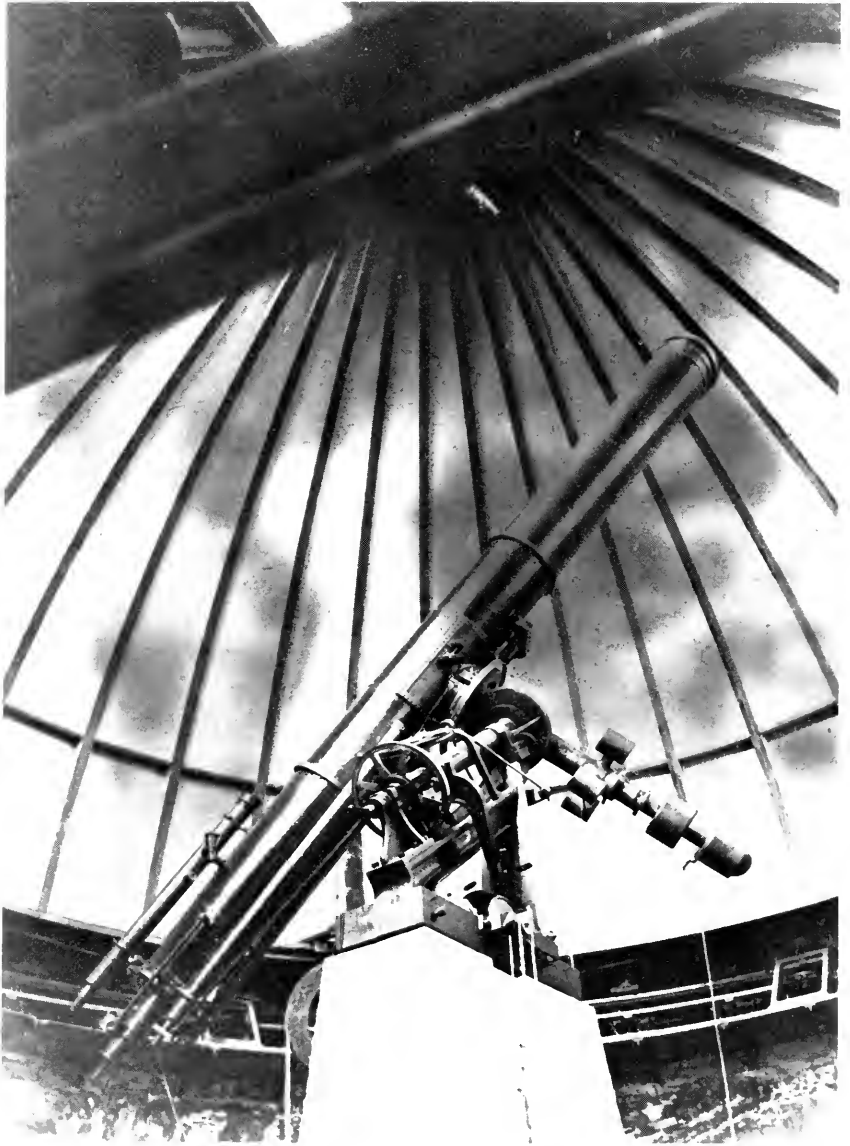
FIGURE 25.—The 12-inch aperture equatorial refracting telescope made by Alvan Clark & Sons for the U.S. Military Academy at West Point. Courtesy U.S. Military Academy Library.
