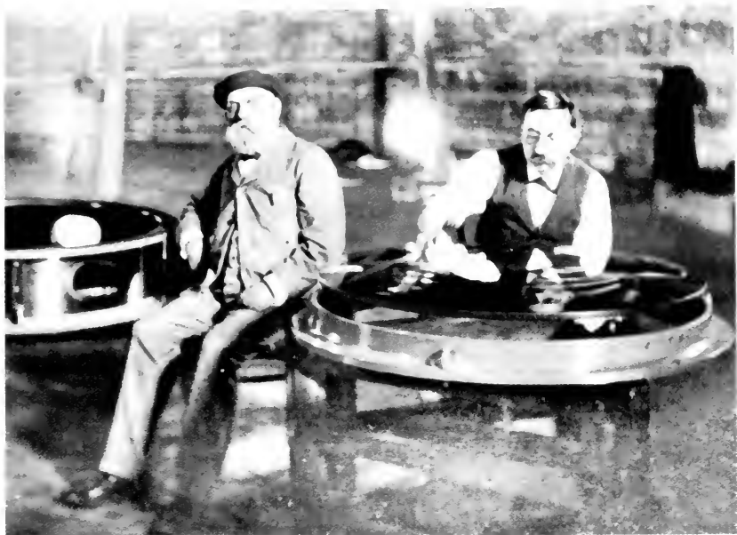
FIGURE 28.—Alvan Graham Clark and Carl A. R. Lundin with the crown glass component of the 40-inch aperture objective lens for the Yerkes Observatory. From George E. Hale, Study of Stellar Evolution (Chicago, 1908), plate xlv.
