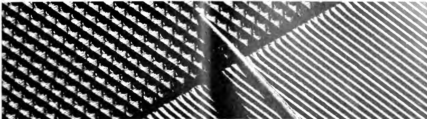
(Above) Extreme close-up contrasting double bastard cut and single cut bastard cut files from the Office of Education film "Fundamentals of Filing" Reviewed in this issue.
