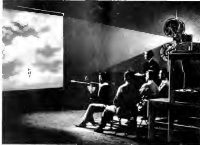
TRAINING UNCLE SAM'S AERIAL GUNNERS is speeded through the use of this new visual device pictured above which utilizes dual 16mm projectors to provide simulated battle conditions for gunnery practice.
