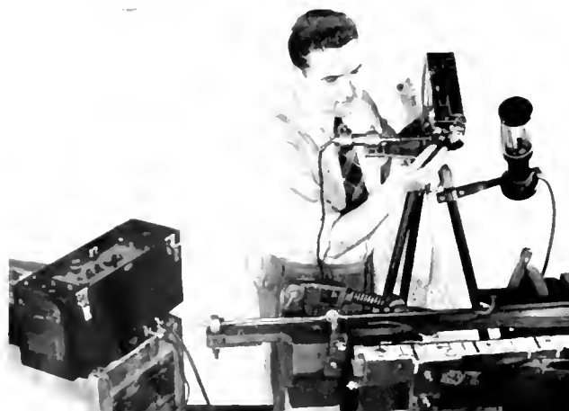
Fig. 12. Eastman Cine-Kodak Special fitted with a stroboscope and setup to make a high-speed record of an action in the operation of a loom.
