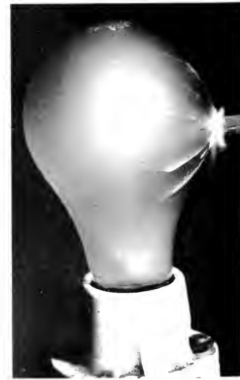
Fig. 4 (Below) Photograph of a 30-caliber bullet (velocity 2700 ft. per sec.) striking an electric lamp bulb. Note that the cracks in the glass travel faster than the bullet. An exposure of less than 2 \times 10^{-6} sec. is required to "stop" the bullet without blur as shown in this picture.
