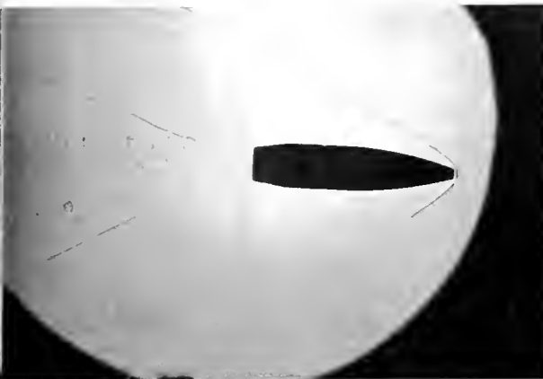
Fig 5 (Top) A microsecond silhouette photograph taken with stroboscopic polarized light to show the stress pattern during the growth of the cracks in a glass plate when violently broken. The crack velocity is 5000 ft per sec. It is measured by taking two photographs spaced in time by 15 microseconds. Fig. 6 (Below) A single-flash silhouette picture of a 50-caliber projectile in flight.
