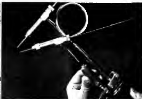
Operator is shown adjusting arc gap in preparation for welding in a typical scene from the new G.E. picture.
