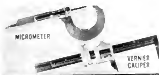
The MICROMETER and the VERNIER CALIPER are both highly accurate measuring instruments. The common ones measure to a thousandth of an inch. Those measuring to a tenth of a thousandth of an inch are coming more and more into use.
