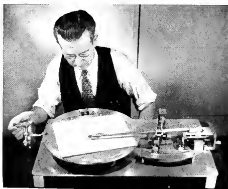
(Above) Norling-designed machine for drawing hairspring animation spirals in Bulova films.
