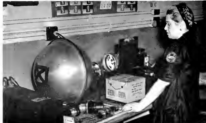
A PERL technician tests the transmission of motion picture lenses.
