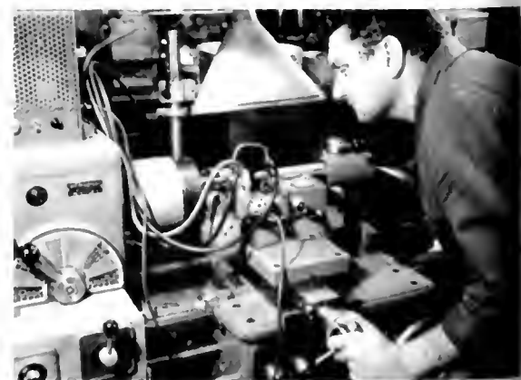
Technician fabricating the pull-down cam for an Arriflex-16 camera, machine operation involves ultra high-speed grinding and precision tracing.
