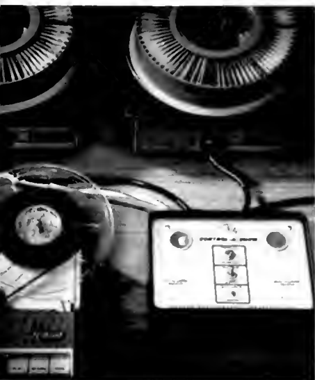
The HPI Control-A-Show mechanism in a Carousel and a stereo tape recorder.
