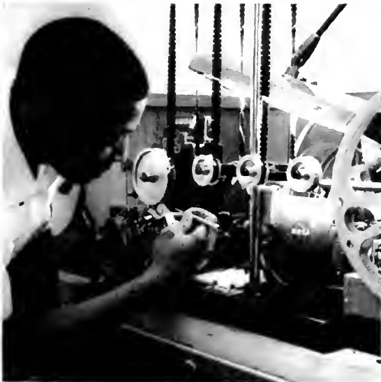
Film technician re-sets edge numbering machine after a new roll of film is threaded. Original film and all prints from the original are given same edge code. Specially fabricated numbering machines place up to seven identifying numbers on the edge of 16mm film. Two of three machines are in continual use, third is for back-up use.
