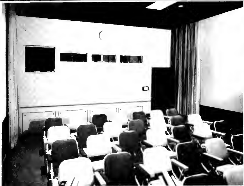
Three tilted glass projection ports, plus a wide viewing window, allow use of full range of equipment. Storage area for tables, chairs is under booth.
