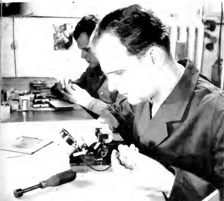
Richter craftsman is shown "tuning up" Arriflex reflex finder shutter on its pre-loaded bearings. Precise mirror-shutter must turn axis, with run-out of less than plus-minus 1/25,000 inches.
