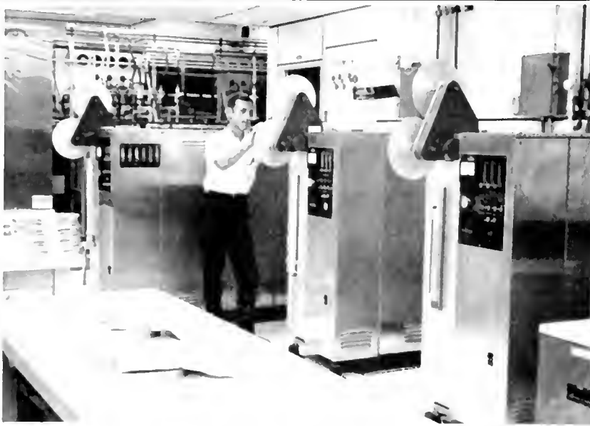
Four motion picture processors serve MSC's Technical Laboratory Branch. Three black and white machines are in the foreground. Over 400,000 feet of color and monochrome motion picture film is processed on these machines each month for the Engineering and Public Affairs Branches at the Center.
