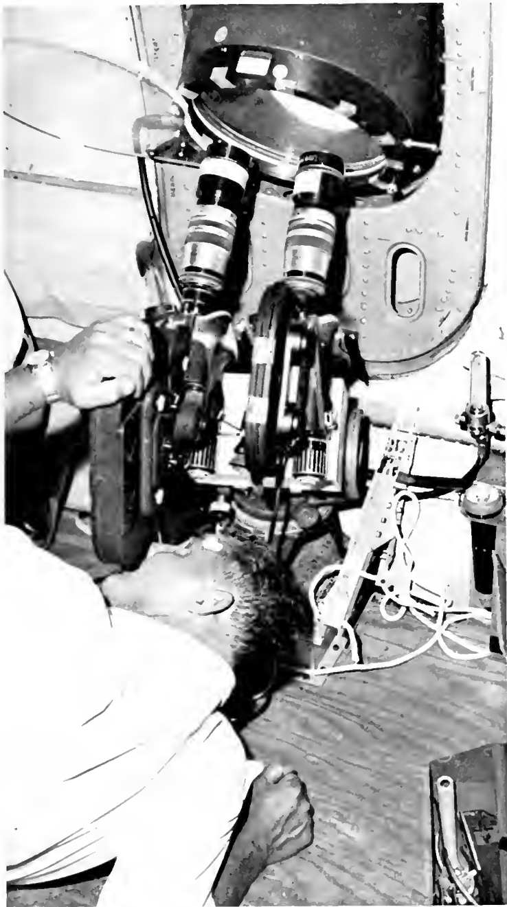
One Arriflex 16s and one Arriflex 16M, both fitted with Kiltitt telephoto lens are dual mounted amidship, positioned to shoot the sun.
