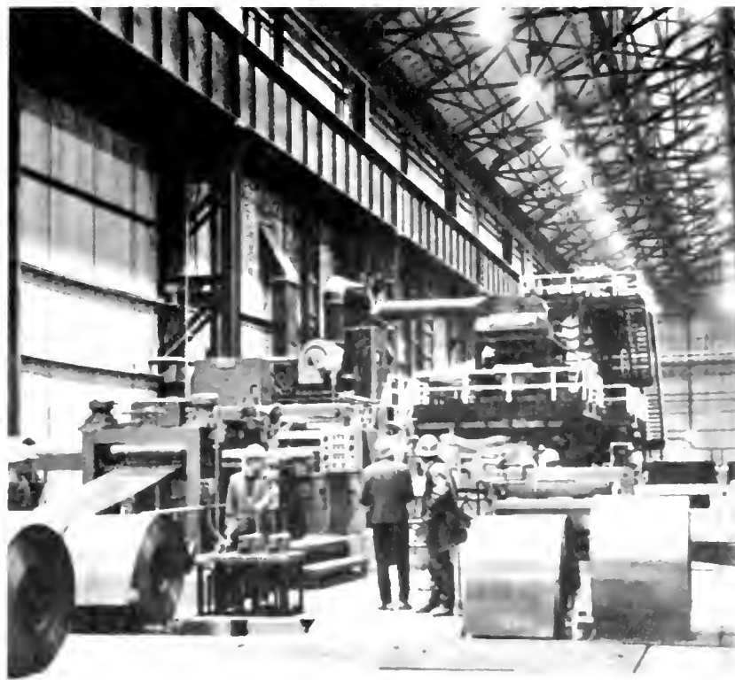
Here steel coils are made ready for entry into Ereğli's electrolytic tinning mill. Template will help meet demands of country's canning industry.
