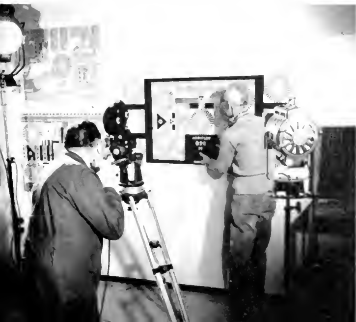
ans put a new Arriflex-16M through final test in this film scene. camera must produce test footage to highest standards of image sharp- picture steadiness before it is permitted to leave the factory.
