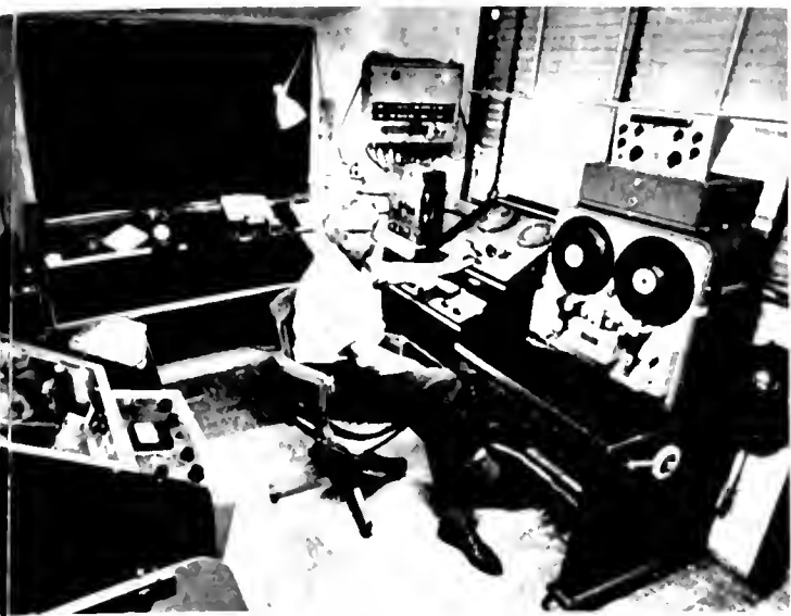
Mixer Raymond Esh handles re-recordings in this transfer room at Wilding. Equipment includes a narration mixer panel and 1/2 inch, 17 1/2 mm magnetic tape and film equipment, provides for transfer from any pair and medium to any other — as well as making optical recordings.
