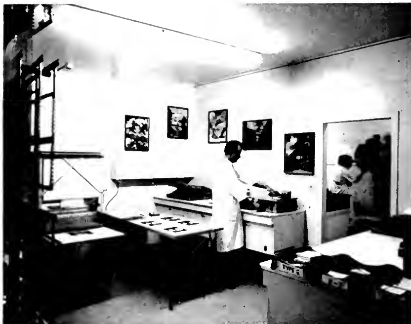
Print drying and mounting room of Photorama: Wilson Tyndal checks a control strip on the Deuschlon, while Jerry Imber adjusts 5X7 Durst enlarger.
