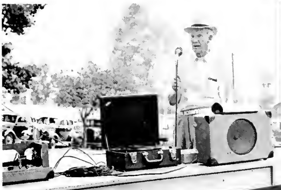
Above: Separate 30 watt amplifier and speaker unit afford portable Public Address facilities for demonstrations, sales meetings, employe assemblies, athletic events, etc.
