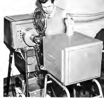
WGS-TV SHOWS FILM PROJECTION via special projector in Chicago setup. GE television film camera, which receives image from the film and "takes" the picture which viewers see, is in foreground.
