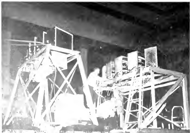
DETAILED REHEARSAL BEFORE MEETING provides an unusually clear view of four corners of the Vitarama screen. One 40-foot scene or five individual panels can be used. Besides 40-foot scenes, lot of the complex projection equipment can be used in a panel show. Absolute steadiness and fine registration are notable features of the Vitarama color visual presentations.
